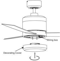
Fig.15 Counterclockwise rotation for opening
