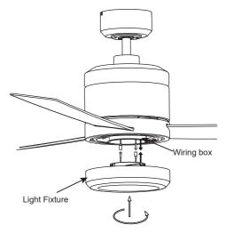
Fig.16 Clockwise rotation for locking
