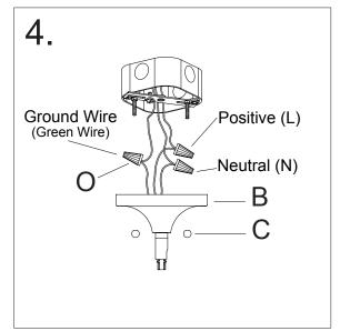
Wire fixture to wires in outlet box. Copper wire is for Ground. Attach canopy to mounting bracket and tighten with ball nuts.
