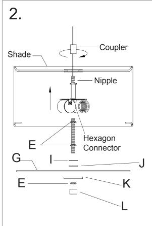
Place shade on the Nipple and tighten with the Coupler. Thread the nipple into Hexagon connector, then secured by hex nut. Put the metal washer and rubber washer on the nipple, adjust them close to the glass diffuser by the hex nut, then put the glass diffuser on the shade spider, and put the Cap close to the glass diffuser, then secured by hex nut and finial.
