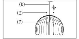
Screw in GU24 light bulb and slide canopy Step.4: back over body.Reattach shade(F) using hexagonal nuts(E).
