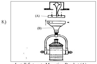
Install fixture to Mounting Bracket (A)
