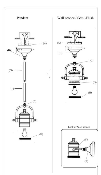
Steps 1 & 2 apply to fixture as a Pendant, Semi-Flush and Wall Sconce. For Pendants contine to Step 3. Wall Sconce and Semi-flush should skip to Step 7
