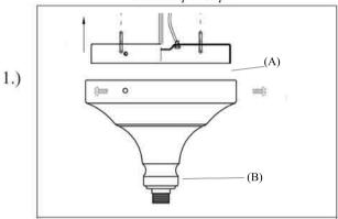
Remove mounting bracket (A) from Canopy (B) to install to electrical box
