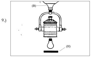
Screw in Lens (H) to cover light Bulb
