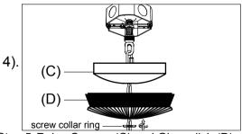
Step.5: Raise Canopy (C) and Glass dish (D) to ceiling and secure with screw collar ring. Install Glass finial (F) at the bottom of the lamp body, Place the Socket cover (G) and Glass Bobeche (H) over the socket and Install light bulb.
