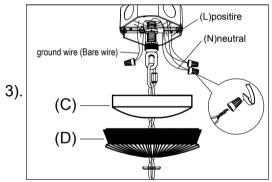
Step.3: Wire fixture to wires in outlet box. Bare wire is for Ground.
