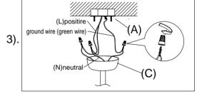
Step.3: Wire fixture to wires in outlet box.
