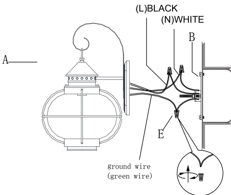
2. Caulk around backplate where fixture meets the wall leave a hole at the bottom to allow water to escape.
