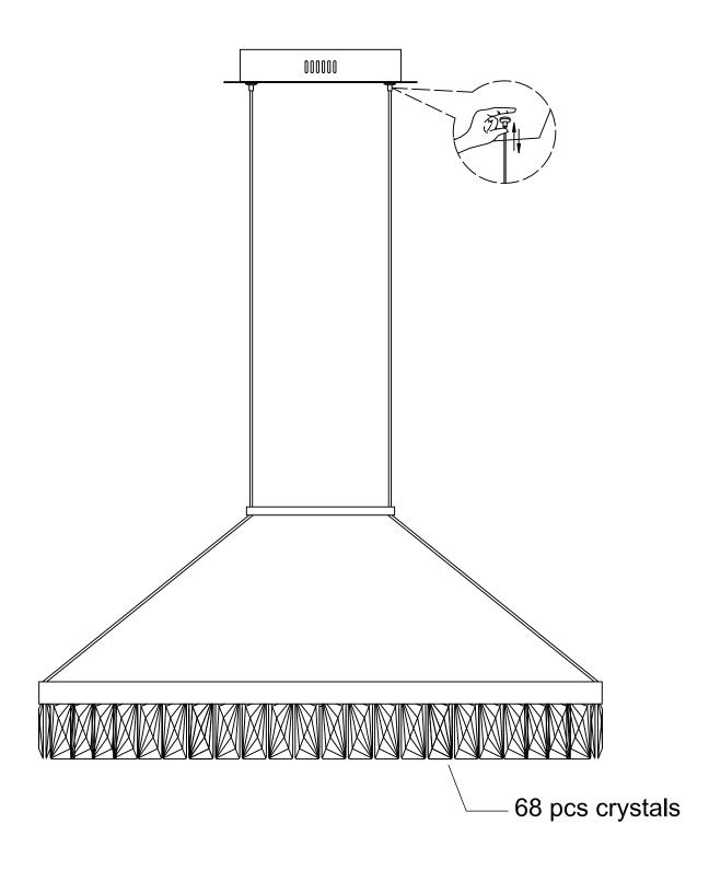
Run crystal along the track at the opening marked. Make space between the crystal when all 68 pieces are attached. 2 extra crystal is provided
