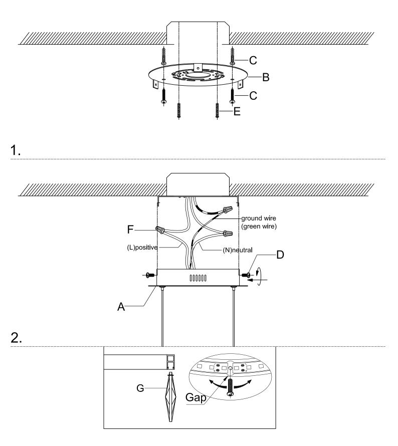
Please refer to the gap mark, insert the crystal (G) into the Aluminum track, then fixed the screw.
