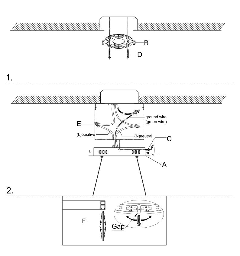
Please refer to the gap mark, insert the crystal (F) into the Aluminum track, then fixed the screw.
