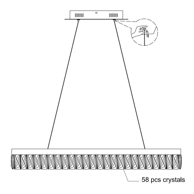
Run crystal along the track at the opening marked. Make space between the crystal when all 58 pieces are attached. 2 extra crystal is provided
