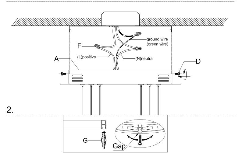
Please refer to the gap mark, insert the crystal (G) into the Aluminum track, then fixed the screw.
