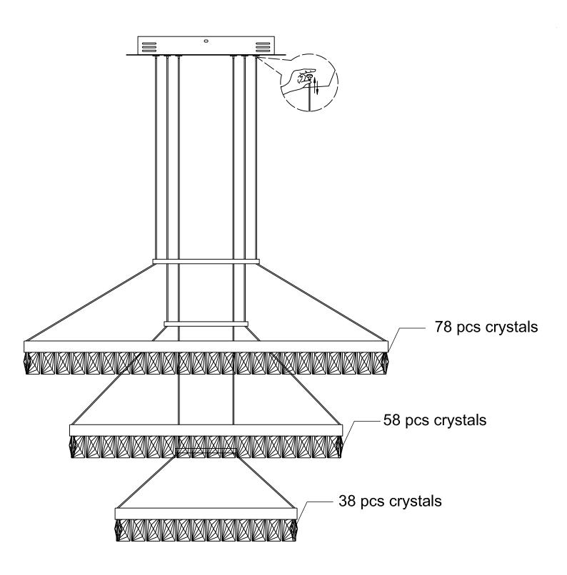
Run crystal along the track at the opening marked. Make space between the crystal when 78 pieces are attached for big one. Make space between the crystal when 58 pieces are attached for middle one. Make space between the crystal when 38 pieces are attached for small one. 6 pcs extra crystal are provided.
