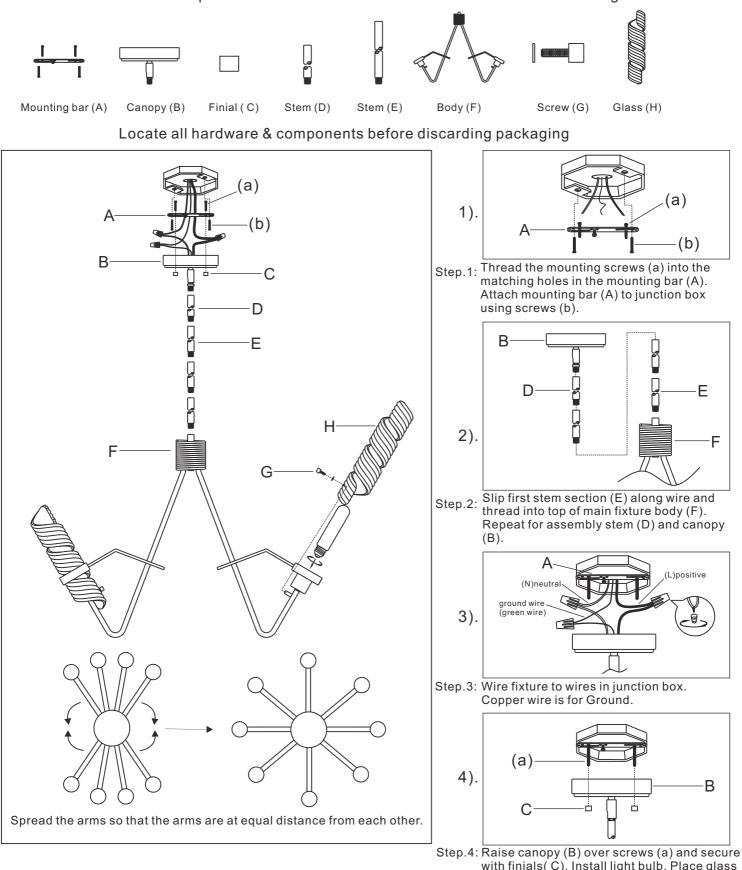
with finials (C). Install light bulb. Place glass (H) over the socket, and then secure glass with screw (G).
