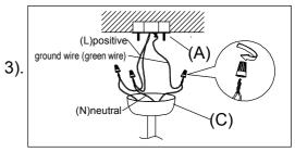
Step.3: Wire fixture to wires in outlet box.
