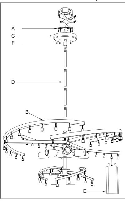
IMPORTANT: For a safe and secure installation, this fixture must be installed by means of support that is independent of the outlet box.
