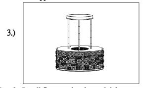
Step.3: Install fixture to bracket and tighten screws at the ends of the canopy (D) to secure.
