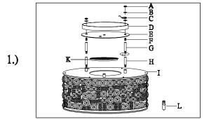
Step.1: Run wire through stems (G&H) as you attach the body (I). Combine stem lengths to meet desired mounting height. Install G9 bulbs (L),
