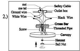
Step.2: Remove mounting bracket from fixture and install to electrical box. Wire fixture to wires in outlet box. Copper wire is for Ground. On wire side
