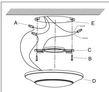
Mounting: These fixtures mount directly to most standard metallic & non-metallic electrical boxes with 2-3/4" to 3-1/2" hole spacingthat are at least 1-1/2" deep. This includes 3-1/2" & 4" octagon boxes, round mud-rings for octagon and square boxes, and 3" & 4"non-metallic round boxes. Products are suitable for mounting on ceilings or walls, and are acceptable for use within closet storage spaces when installed per NEC requirements.
