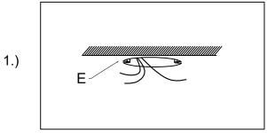
Step 1. Bring positive, neutral, and ground supply conductors (120V, 60Hz) to the room side from junction box(E).
