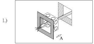
Step.1: Fix the Mounting box(B) to the hole.
