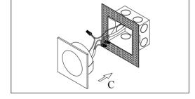
Step.3: Caulk around the housing with silicone sealant to prevent water intrusion.
