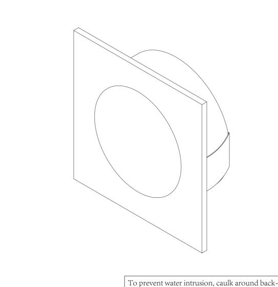
To prevent water intrusion, caulk around back-plate where fixture meets the wall using outdoor silicone sealant. Leave a small gap at the bottom to allow moisture to exit.
