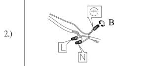
Step.2: Wire fixture to wires in outlet box. Green/Copper wire is for Ground.
