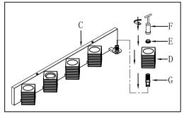
Step.4: Install G9 LED bulb(G) into socket, Position Glass(D) onto the socket of fixture body(C), then secure with socket ring(E) with Glass (D) onto Fixture body(C) by using spanner(F).
