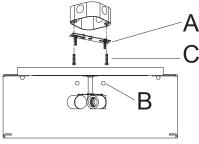
Remove mounting bracket from fixture and install to electrical box.
