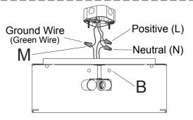
Wire fixture to wires in outlet box. Copper wire is for Ground. Attach canopy to mounting bracket and tighten with ball nuts.
