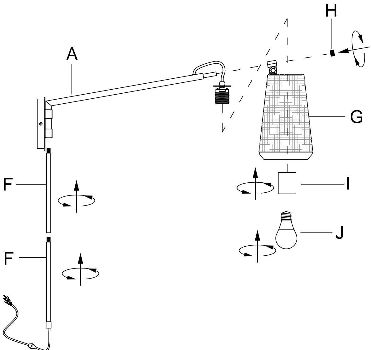
**1.** Don't connect wire in back plate , use the plug to plug into a power outlet
