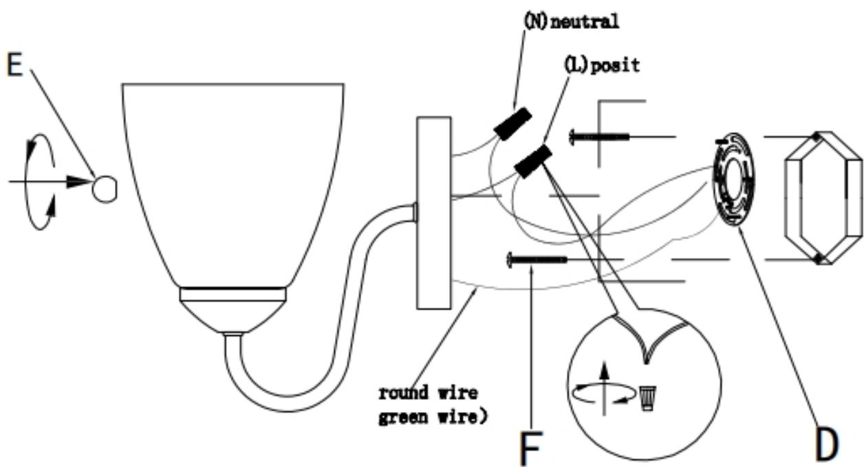
1. Install the Mounting Bracket ( D ) to electrical box.
