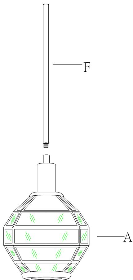
1. Run wire through stems and combine stem lengths to meet desired mounting height.
