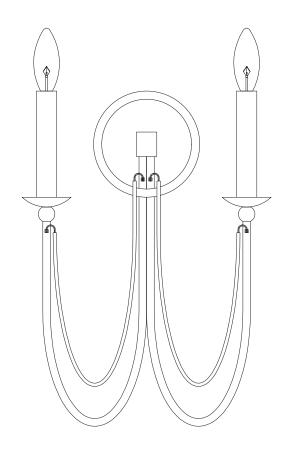
Lamping | Ampoule: 1 × E12 Medium Base 60W (Not Included)
