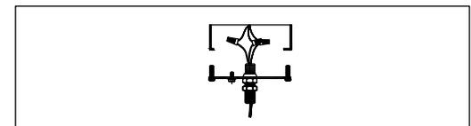
Step.4: Wire fixture to wires in outlet box. Copper/Green wire is for Ground. Pull canopy through screw ring (E) up chain to ceiling and tighten securely.
