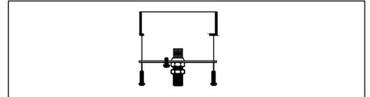
Step.1: Remove mounting bracket from fixture and install to electrical box.
