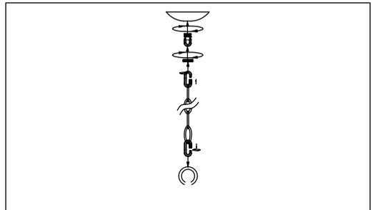
Step.3: Remove ring from top and slide down chain. Place canopy (D) onto chain (C) and let slide to top of fixture. Install nipple and cross bar into top of chain loop.
