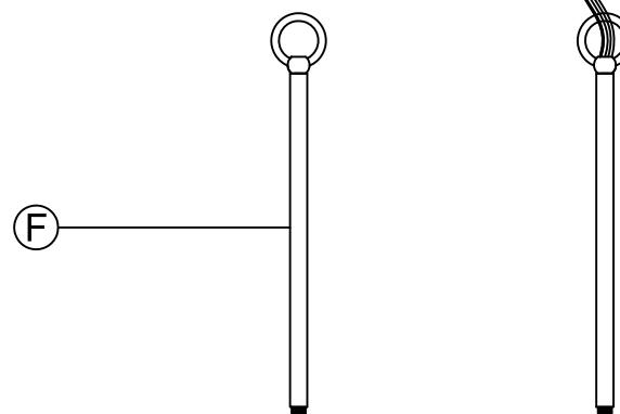
Install stem to center Fixture and attach appropriate amount of chain to loop to achieve desired mounting height. Thread wire through every 3rd loop of chain
