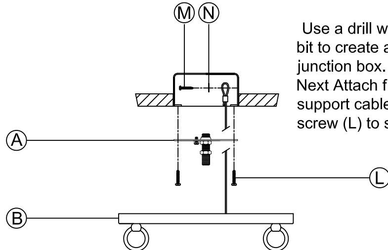
Use a drill with a #29 ( $\varnothing.136$ ) (3.5mm) bit to create a mounting hole in the junction box.
