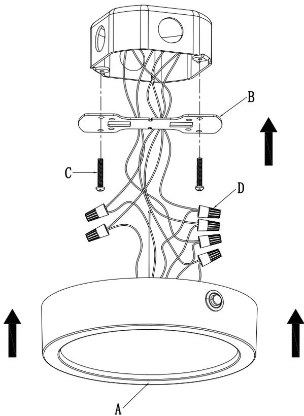
1. Prior to installation, install the mounting plate on the junction box with mounting screws. Drive screws completely to the end of the junction box.
