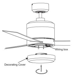
Fig.16 Clockwise rotation for locking
