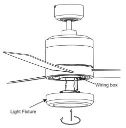
Fig.15 Counterclockwise rotation for opening
