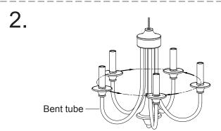
Rotate the bent tube to the suitable position.
