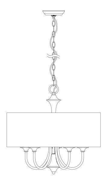
Lamping | Ampoule: 5 x E12 60W ( Not Included )
