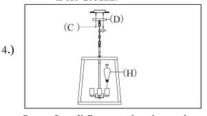
Step4:Install fixture to bracket and tighten screws at the ends of the canopy to secure.then install the bulb(H)
