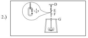
Step.2: Install top loop E to center stem and attach appropriate amount of chain to loop to achieve desired mounting height.
