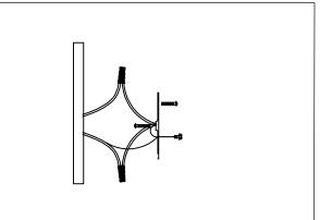
1.Remove mounting bracket from fixture and install to electrical box. Then wire fixture to wires in outlet box. Copper wire is for Ground.
