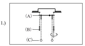
Step1:Remove mounting bracket from fixture and install to electrical box.
