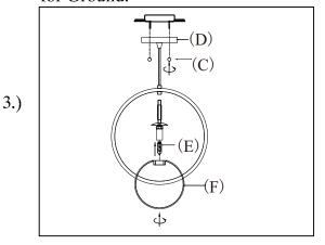
Step3: Install fixture to the bracket using ball nuts on the canopy. Install bulb provided into socket and thread the glass onto socket.
