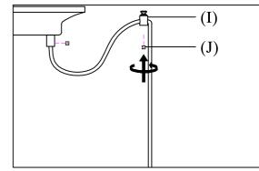
Step2: Adjust wire length to desired mounting height, and tighten strain relief screws to secure.
