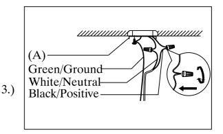
Step3: Wire fixture to wires in outlet box. Green wire is for Ground.
