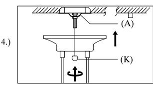
Step4: Install fixture to bracket and Ball Nuts at the ends of the canopy to secure.
