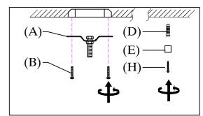
Step1: Use 3/8" drill bit to attach anchors (D) to ceiling. Hold iron accessory (E) over the anchor and secure using mounting screw (H).
