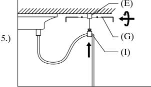
Step5: Load the line fixing device (I) into the iron accessory (E), adjust the angle of the wire, and use the inner hexagon wrench (G) to lock the screw.
