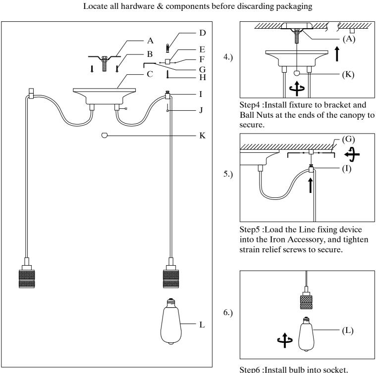
Step6: Install bulb into socket.
