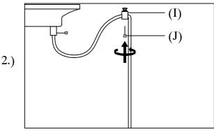
Step2: Adjust wire length to desired mounting height, and tighten strain relief screws to secure.
