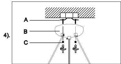
Step.4: Adjust cable through separator to desired hanging height and tighten strain relief screws at top and bottom to secure. Refer to lamp installation to hang shades from cable.
