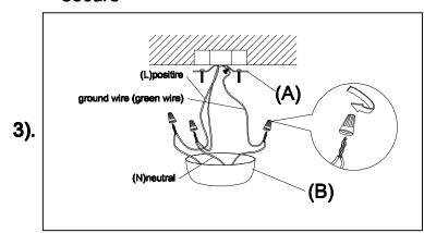
Step.3: Wire fixture to wires in outlet box. Green wire is for Ground.
