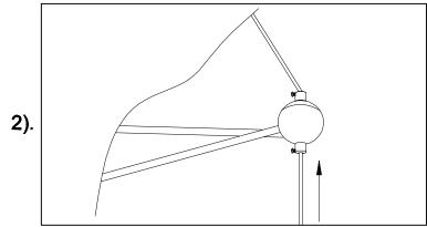
Step.2: Adjust cable length to desired mounting height, and tighten strain relief screws to secure
