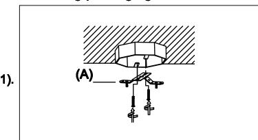
Step.1: Remove mounting bracket(A) from fixture and install to electrical box.
