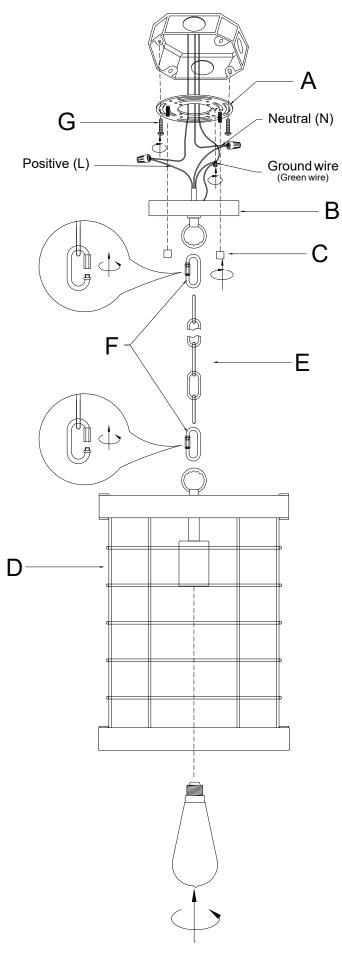
Attach appropriate amount of chain to loop to achieve desired mounting height. Thread wire through every 3rd loop of chain. Remove ring from loop and slide down chain. Place canopy onto chain and let slide to top of fixture. Install nipple and cross bar into top of chain loop.
