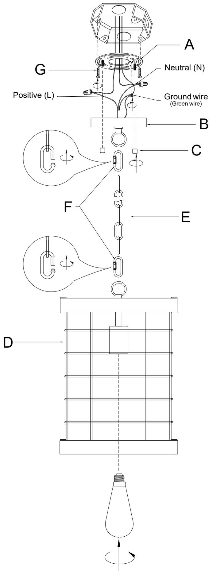
Attach appropriate amount of chain to loop to achieve desired mounting height. Thread wire through every 3rd loop of chain. Remove ring from loop and slide down chain. Place canopy onto chain and let slide to top of fixture. Install nipple and cross bar into top of chain loop.
