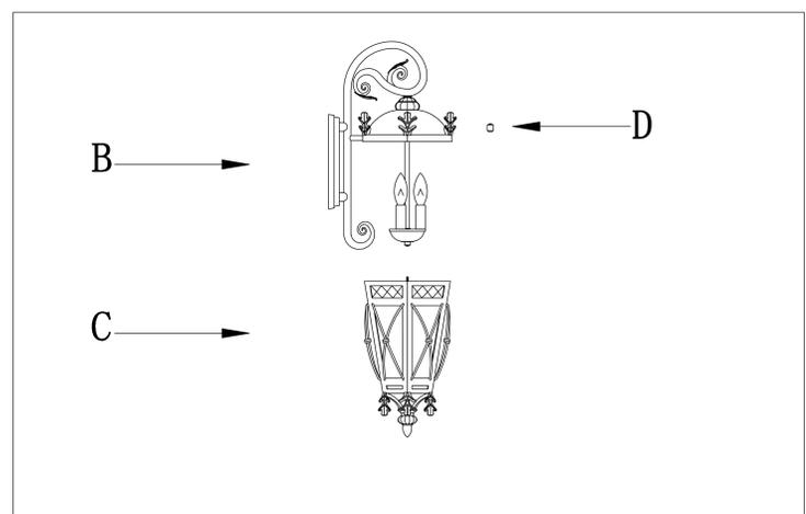
Step.4: Attach cage(C) to fixture , using cylinder knob(D) at screws.
