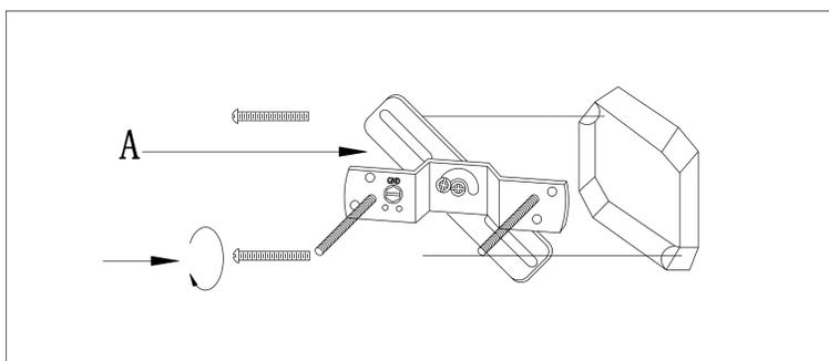
Step.1: Remove mounting bracket from fixture(B) and install to electrical box. then wire fixture to wires in outlet box. Copper wire is for Ground.
