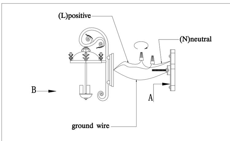
Step.2: Attach back plate to mounting bracket and tighten ball nuts so fixture meets wall. Caulk fixture where back plate meets the wall with silicone sealant.
