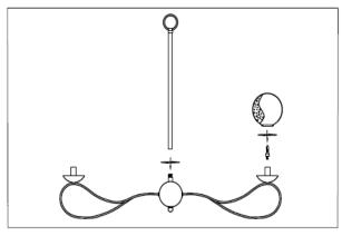
1. Run wire through center stem and attach to the body of the fixture.
