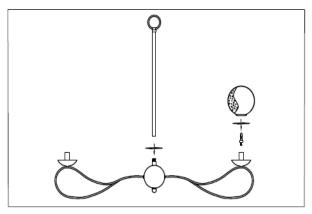
1. Run wire through center stem and attach to the body of the fixture.
