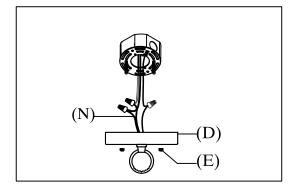
step3:Wire fixture to wires in outlet box. Copper wire is for Ground. Attach canopy to mounting bracket and tighten with ball nuts.
