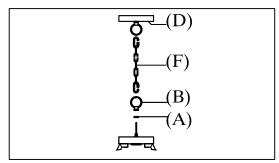
step1:Thread wire through the plate cap, the loop, and every 3rd loop of chain, and the canopy.
