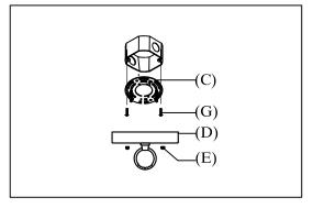
step1: Remove mounting bracket from canopy and install to electrical box.
