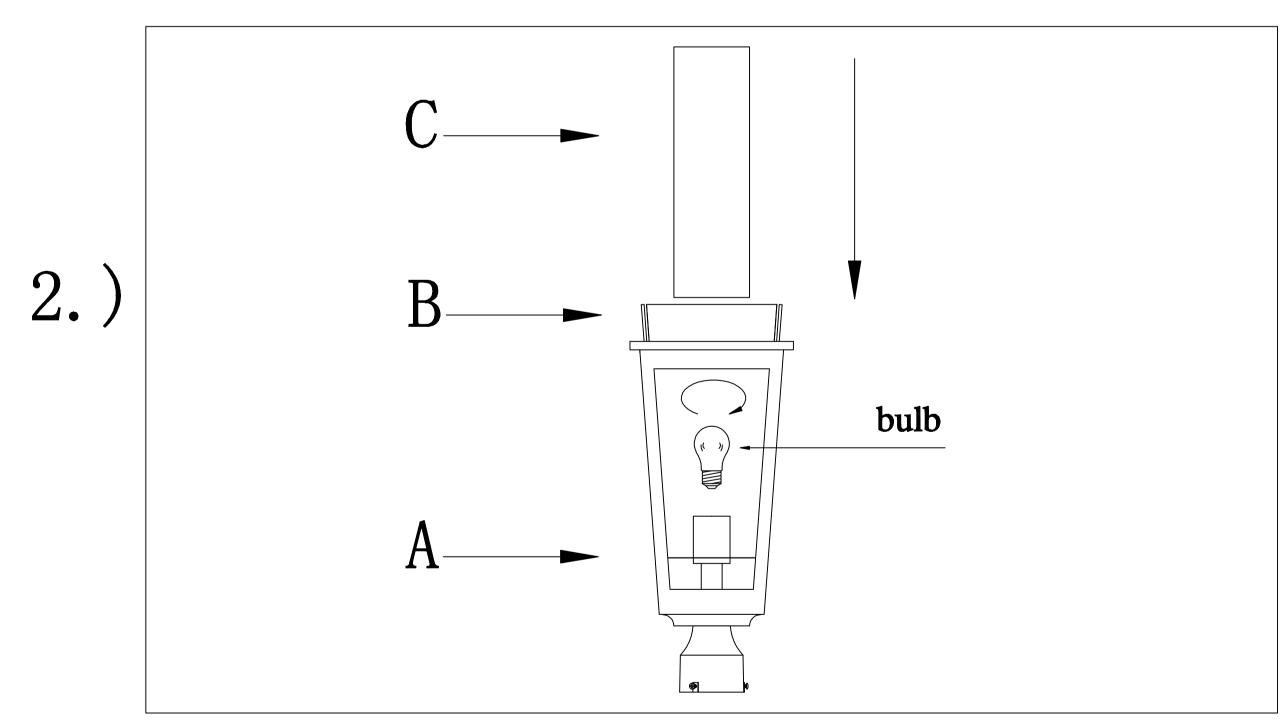
Step.2: Install MB bulb. Slide four clear glass(B) into fixture(A), and then slide frosted glass(C) into fixture(A).
