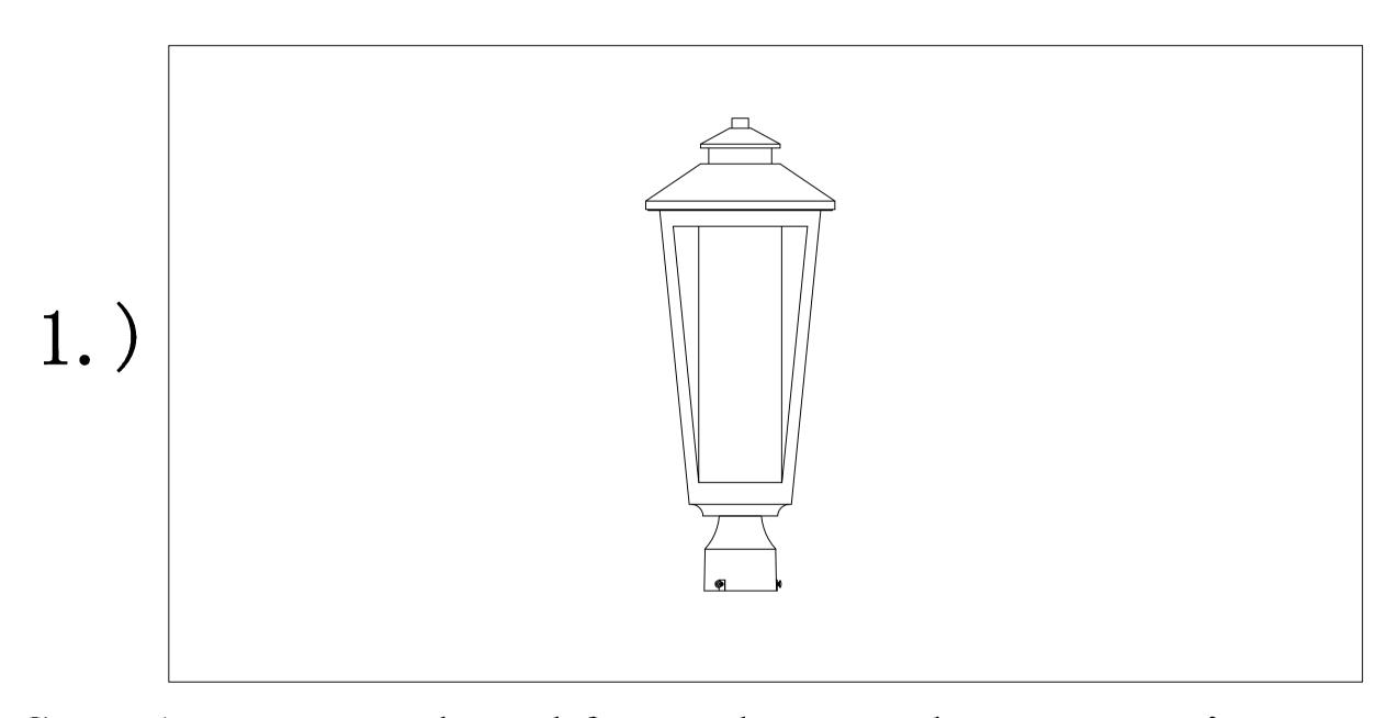
Step.1: Remove hood from the post by unscrewing top finial and two screws within the hood.
