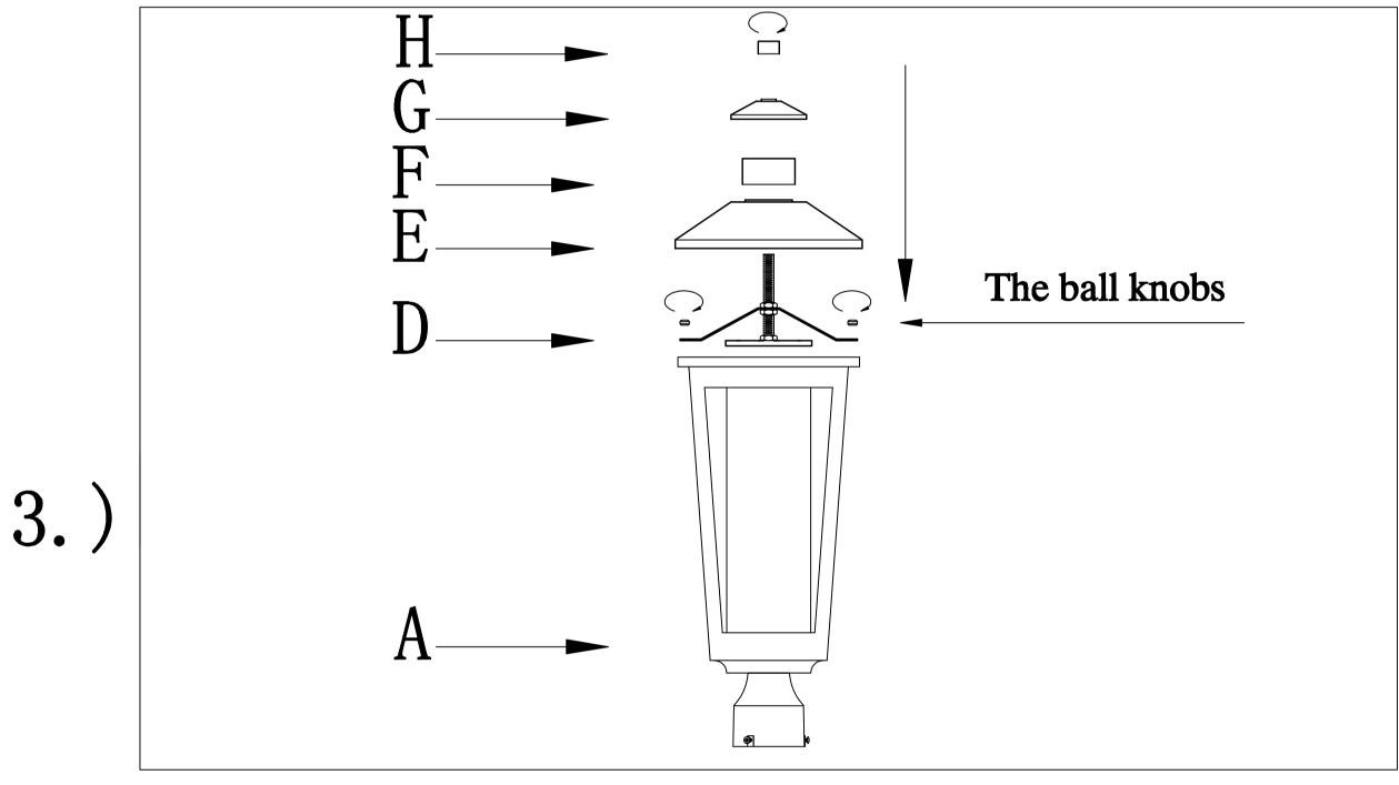
Step.3: Attach harp (D) to fixture, using ball nuts. Run the hood(E), neck(F), top cover(G) over the threaded tube, then tighten the finial (H).
