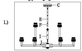
Step.1: Threaded the center stem(I) to the Coupler(J) until it is secured.
