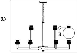
Step3: Placed the Glass(H) on the socket, then secured by socket ring(G)
