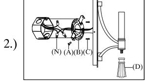
Step 2: Wire fixture to wires in outlet box. Copper wire is for Ground. Attach wall sconce to mounting bracket and secure using screws (A) provided. Finally attach glass finial(D).
