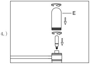
Step.4: Install 40 Watt candelabra base bulb. Then, Thread glass (E) into fixture.
