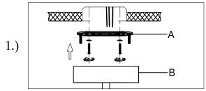
Step.1: Remove mounting bracket (A) from canopy (B) and install to electrical box.
