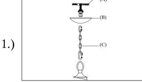
Step 1: Weave the fixture wire through every 3rd link in the chain and canopy. Connect the chain to the top loop on fixture and screw collar loop on canopy by using loop lock.
