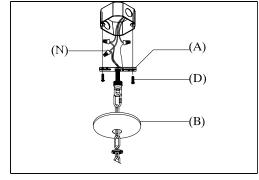
Step 2: Attach the mounting strap (A) to the outlet box by using mounting screws (D). Make wire connections using wire nuts (N), and attach the fixture grounding wire to the mounting strap with the green grounding screws. Attach the canopy to the mounting strap and secure it with the screw collar.
