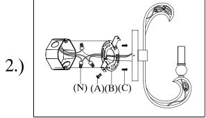
Step 2: Wire fixture to wires in outlet box using wire nuts (N). Copper wire is for Ground. Attach wall sconce to mounting bracket and secure using screws (A) provided.
