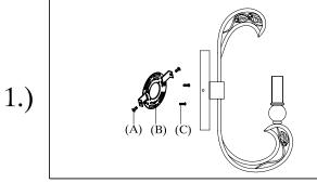
Step 1: Remove mounting bracket(B) from fixture and install to electrical box using mounting screws(C).
