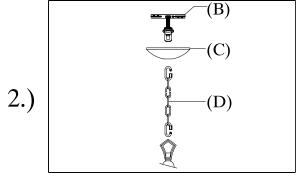
Step 2: Weave the fixture wire through every 3rd link in the chain and canopy. Connect the chain to the top loop on fixture and screw collar loop on canopy by using loop lock.
