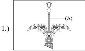
Step 1: Attach the center rod (A) to the fixture.
