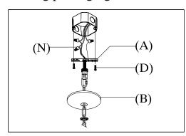
Step 3: Attach the mounting strap (A) to the outlet box by using mounting screws (D). Make wire connections using wire nuts(N), and attach the fixture grounding wire to the mounting strap with the green grounding screws. Attach the canopy to the mounting strap and secure it with the screw collar.
