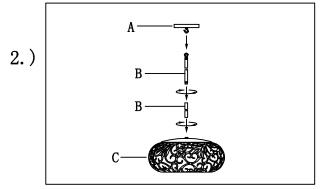
Step. 2: Run wire through stems(B) and combine stem lengths to meet desired mounting height.
