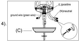
Step.4: Wire fixture to wires in outlet box. Green wire is fo Ground.
