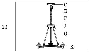
Step1: Carefully remove packaging from fixture. Run wire through stems (E)&(F) and combine stem lengths to meet desired mounting height. Then attach canopy (C) to fixture.
