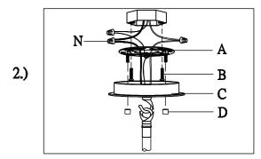
Step2:Remove mounting bracket(A) from canopy. Install fixture to bracket and tighten ball nuts(D) on the canopy to secure.
