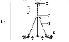
Step1: Carefully remove packaging from fixture. Run wire through stems (E)&(F) and combine stem lengths to meet desired mounting height. Then attach canopy (C) to fixture.
