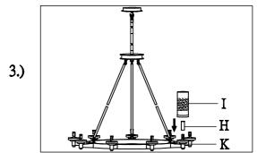
Step3: Attached the Candle tube(H) and Glass(I) onto the Cup(K)
